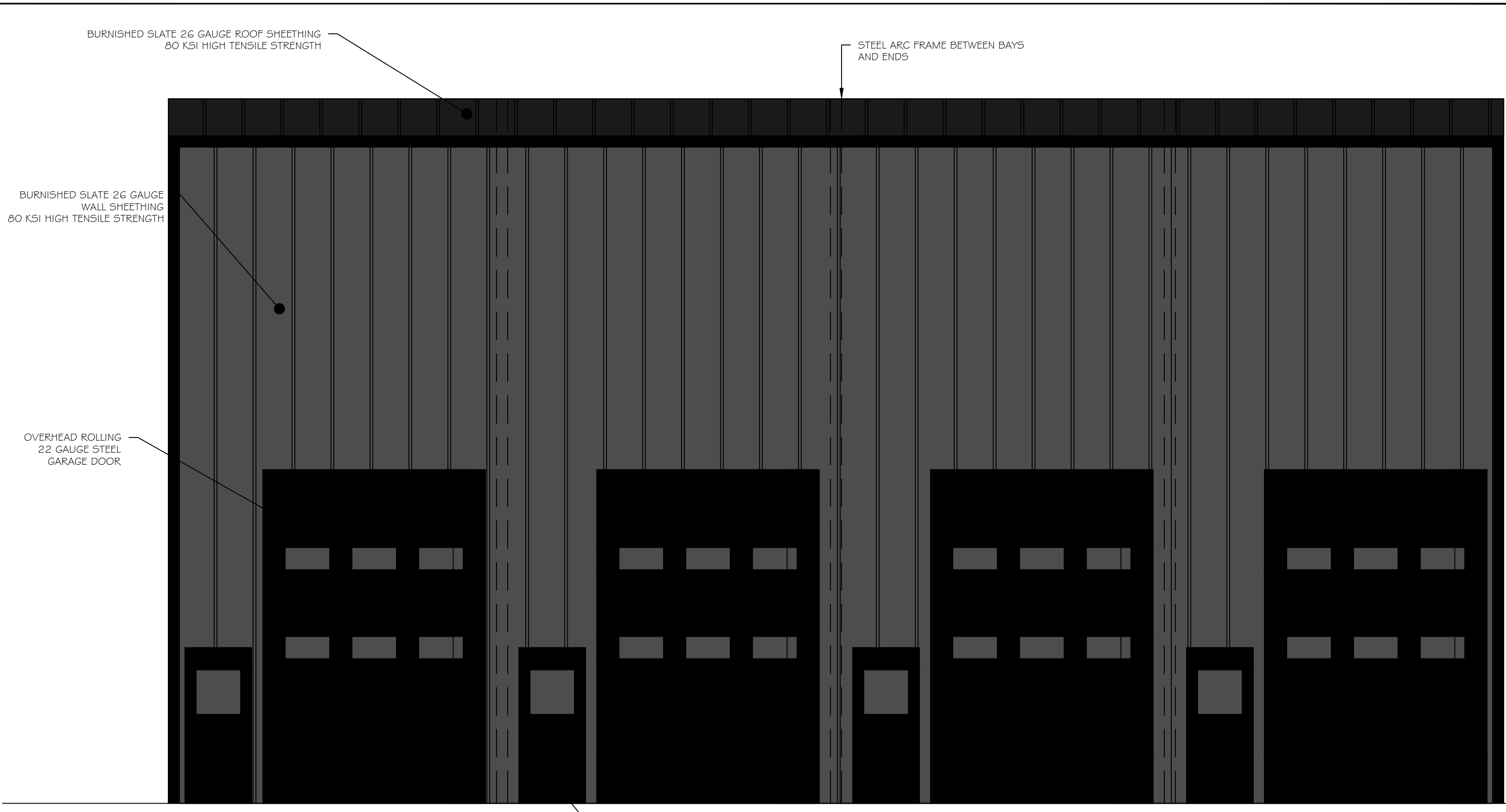
4-BAY WAREHOUSE FRONT ELEVATION 1/4"=1'-0"
