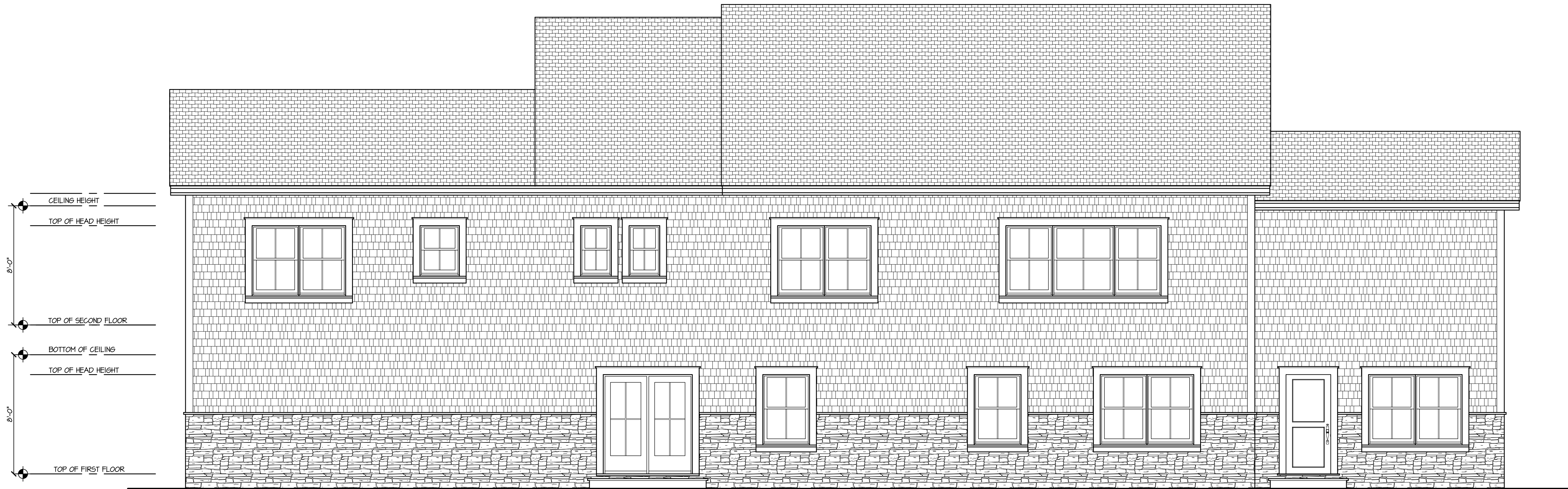
1 PROPOSED REAR ELEVATION SCALE: 1/4"=1'-0"
