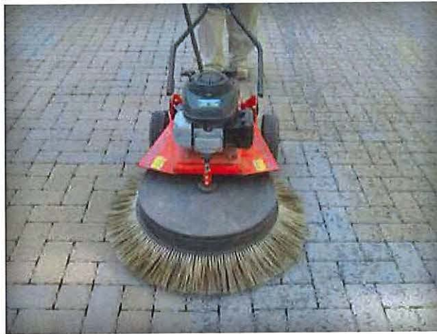
Figure 16. Rotary brushes increase cleaning efficiencies.
