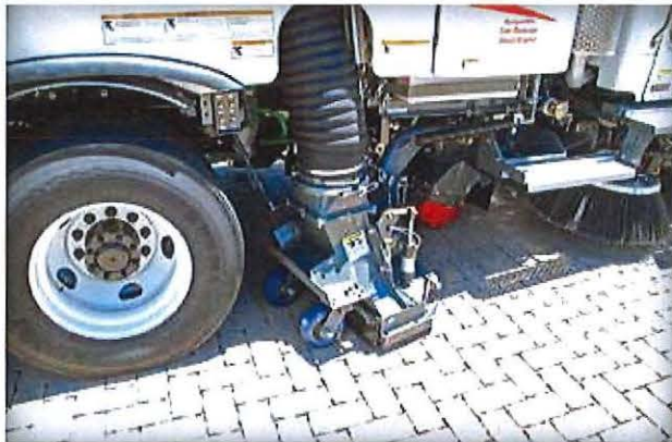
Figure 22. A true vacuum machine cleaning neglected PICP.
