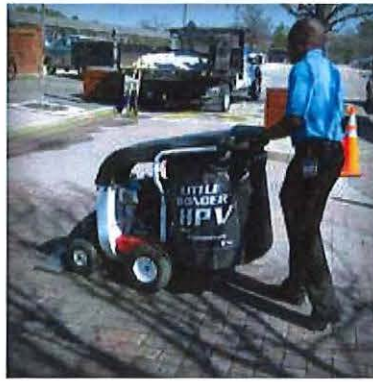
Figure 18. Walk-behind vacuum cleans a small parking area.
