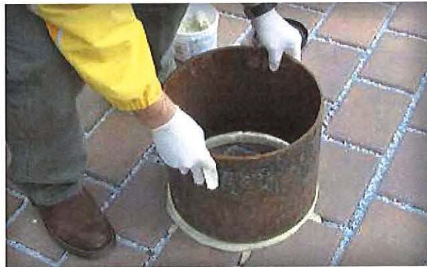
Figure 12. Steps in setting up test equipment for measuring surface infiltration using ASTM C1781.
