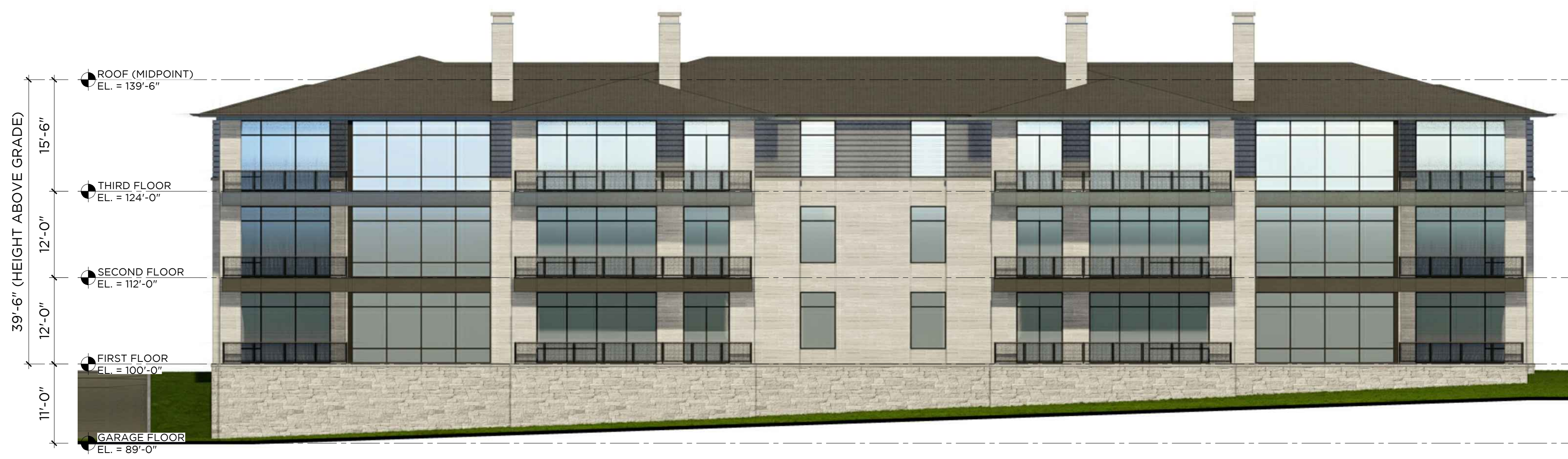
1 WEST ELEVATION 12-UNIT; COLOR SCHEME 'SAND' 3/32" = 1'-0"
