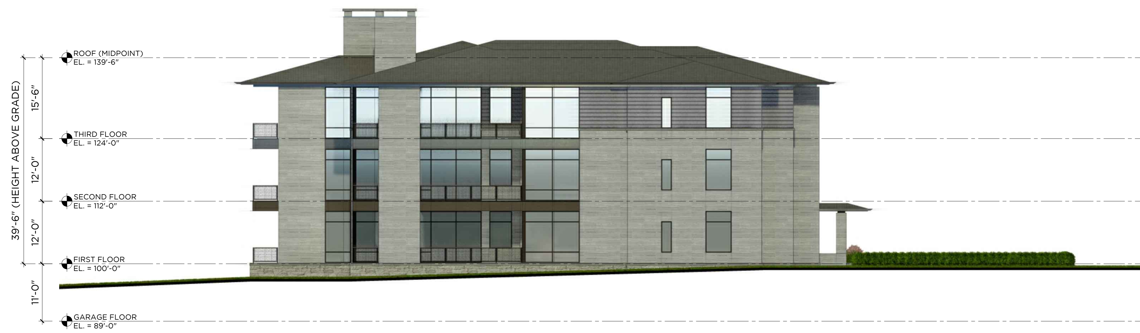
3 SOUTH ELEVATION 12-UNIT: COLOR SCHEME 'SLATE' 3/32" = 1'-0"
