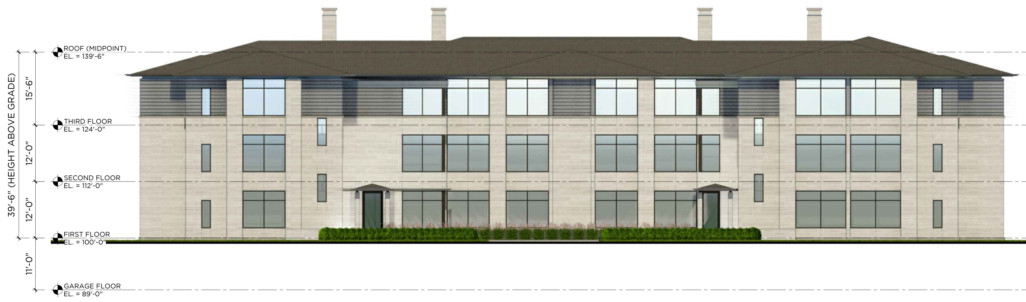
1 EAST ELEVATION 12-UNIT; COLOR SCHEME 'SAND' 3/32" = 1'-0"
