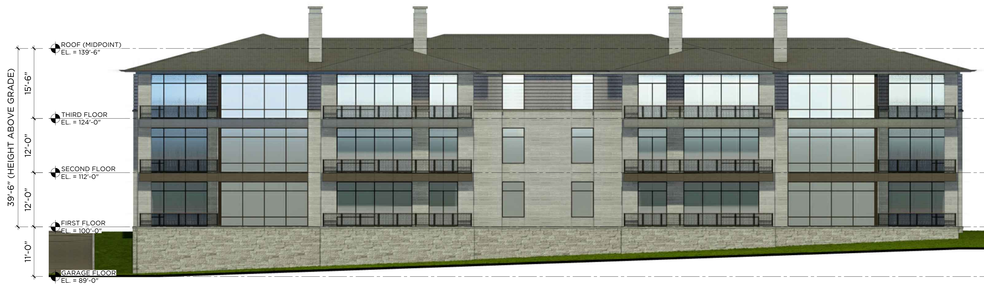
3 WEST ELEVATION 12-UNIT; COLOR SCHEME 'SLATE' 3/32" = 1'-0"
