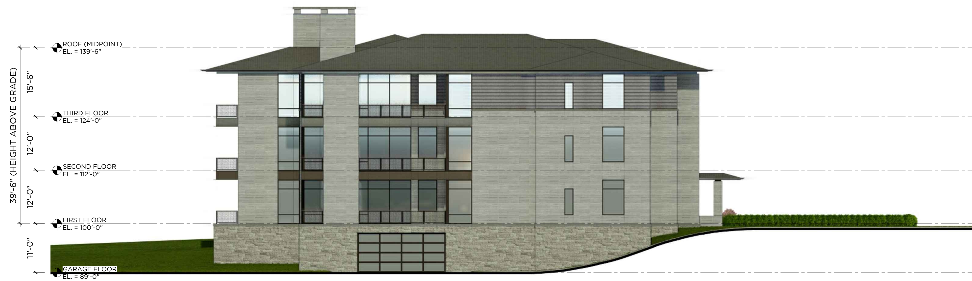
3 SOUTH ELEVATION 12-UNIT: COLOR SCHEME 'SLATE' 3/32" = 1'-0"
