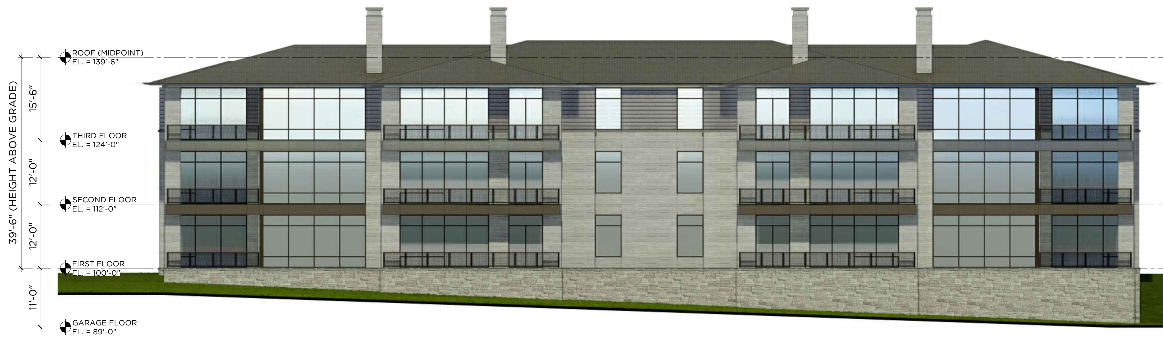
3 WEST ELEVATION 12-UNIT; COLOR SCHEME 'SLATE' 3/32" = 1'-0"
