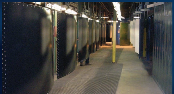
▲ Glass-fused-to-steel panels on the production line.
