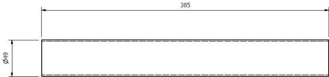
Figure 2.8b Quartz Sleeve Detail for the WF-125-6 and the WF-225-8. All dimensions in mm. (Source: ATG)
