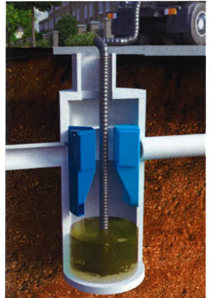
Fig.5 Sediment is removed with a vactor hose (First Defense model FD-4, shown).
