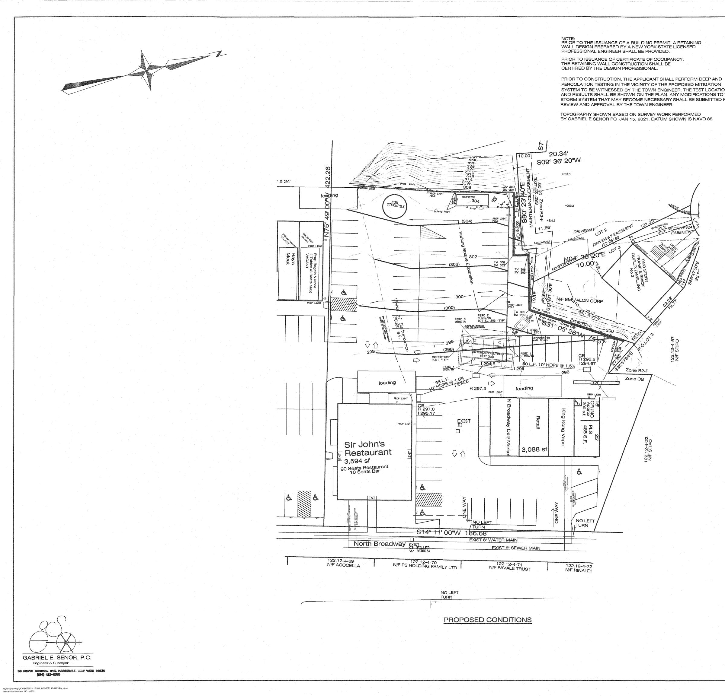
PERCOLATION TESTING IN THE VICINITY OF THE PROPOSED MITIGATION SYSTEM TO BE WITNESSED BY THE TOWN ENGINEER. THE TEST LOCATIONS AND RESULTS SHALL BE SHOWN ON THE PLAN, ANY MODIFICATIONS TO THE STORM SYSTEM THAT MAY BECOME NECESSARY SHALL BE SUBMITTED FOR
