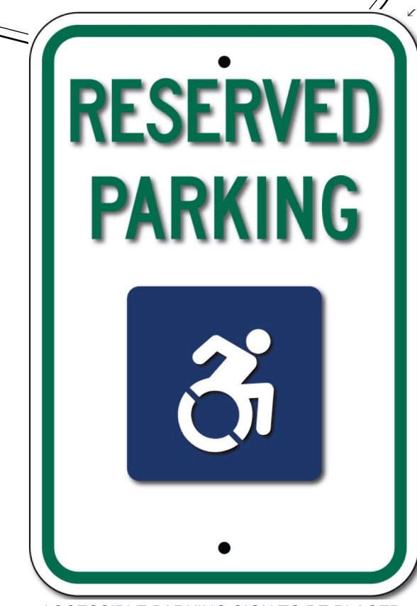
ACCESSIBLE PARKING SIGN TO BE PLACED AT THE FRONT OF EACH ACCESSIBLE SPACE. ACCESSIBLE ICON TO BE PAINTED IN EACH ACCESSIBLE PARKING SPACE.
