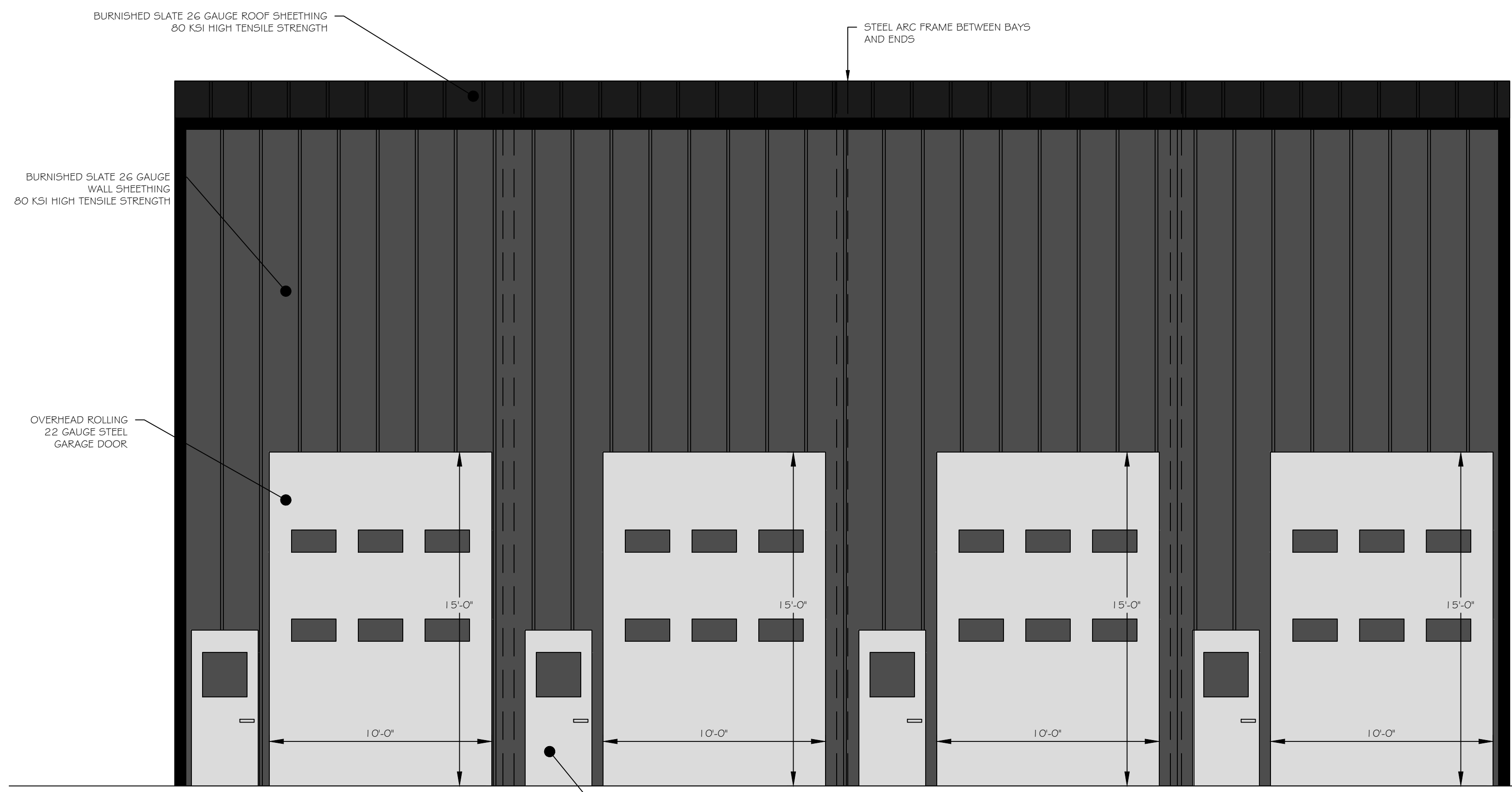
4-BAY WAREHOUSE FRONT ELEVATION
