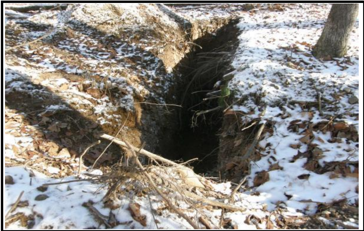
Photo 25: One of many deep percolation test pits located throughout project area. View to east.
