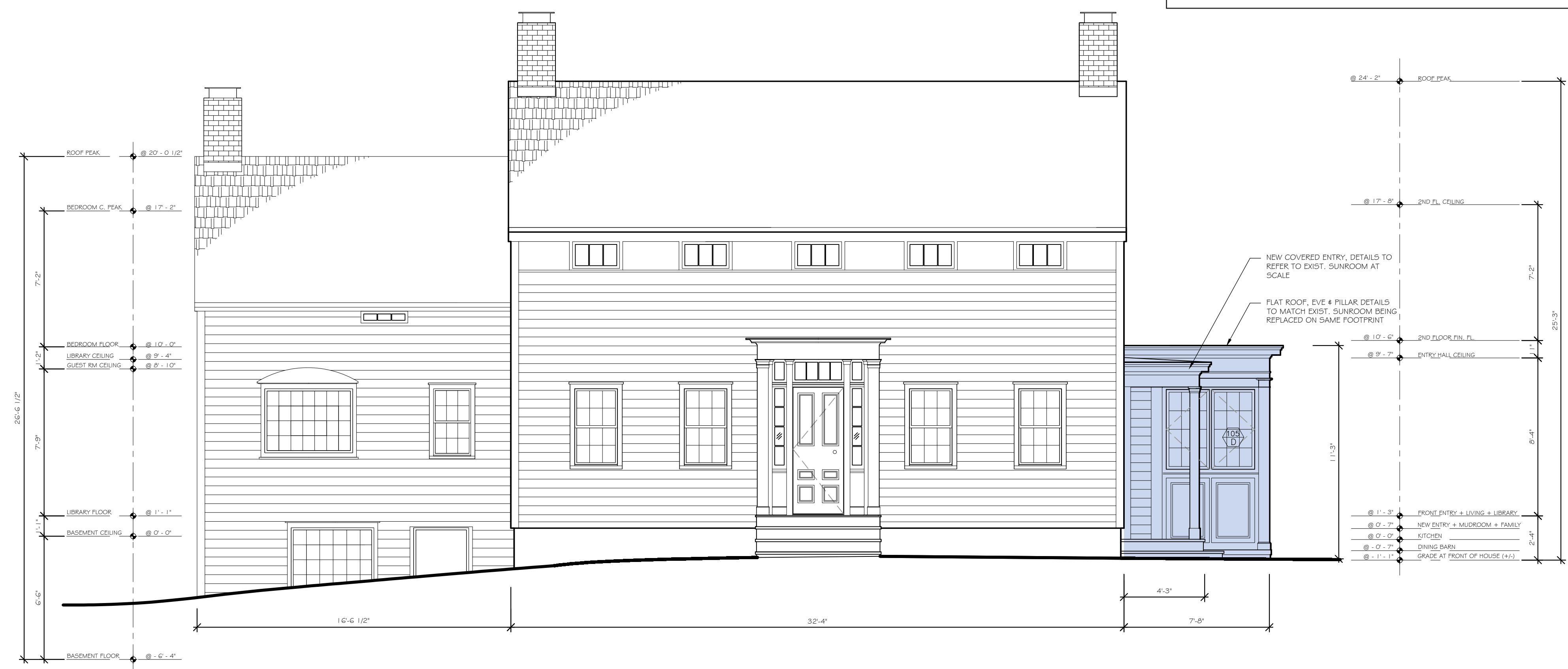
2 PROPOSED SOUTH / FRONT ELEVATION SCALE: 1/4" = 1'-0"
