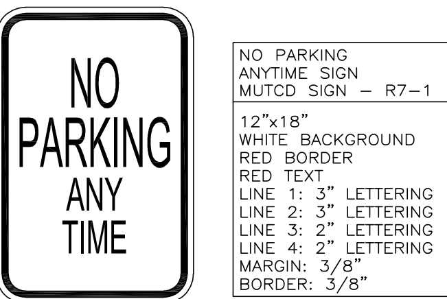
NO PARKING ANY TIME SIGN DETAIL N.T.S.
