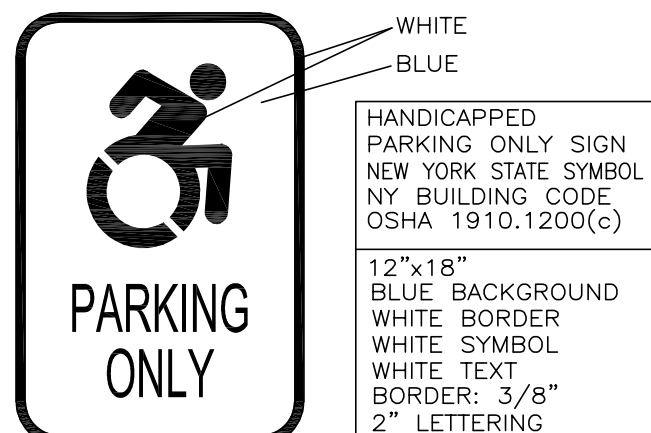
ACCESSIBLE PARKING ONLY SIGN DETAIL N.T.S.
