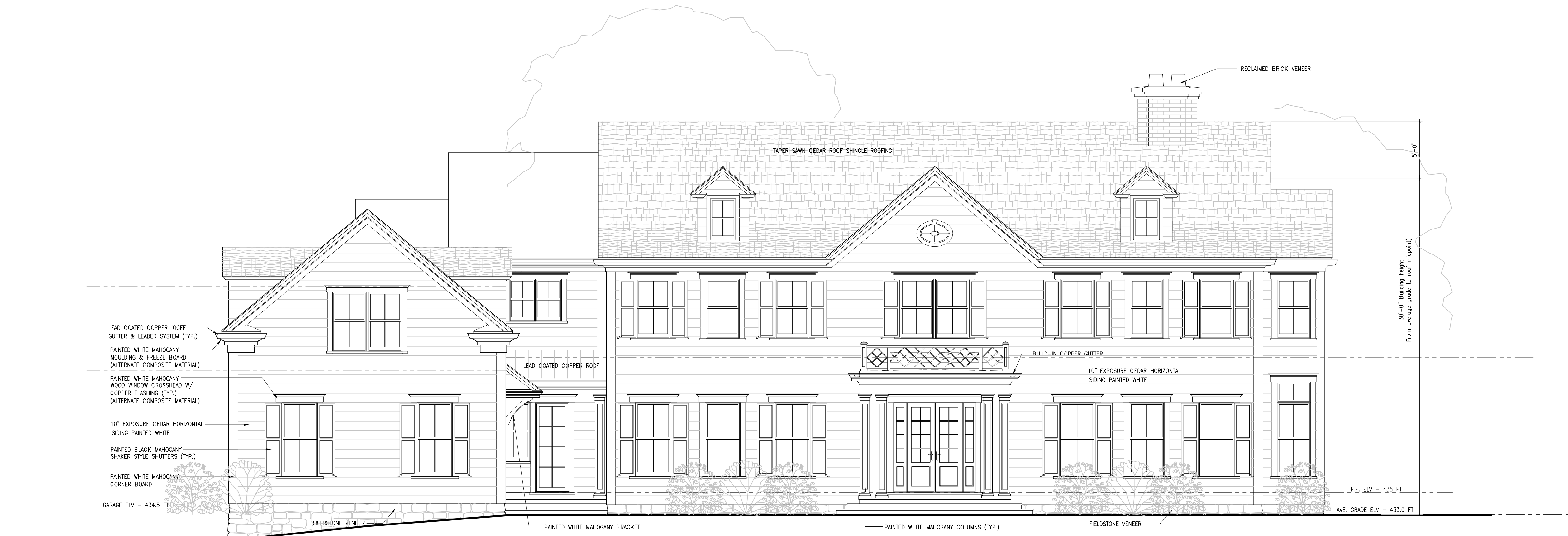
1 PROPOSED FRONT ELEVATION Scale: 3/16" = 1'-0"
