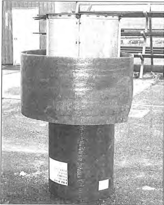
Fig 1. Upside down inlet and screen.
