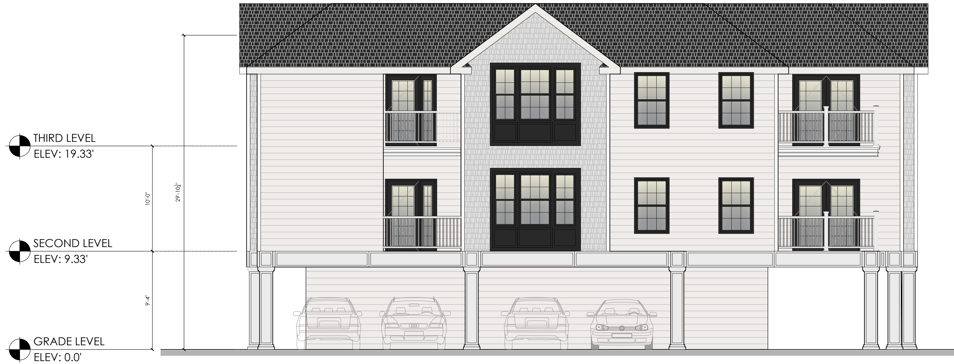
1 ELEVATION - SIDE (BLDG A) SCALE: 3/16" = 1'-0"
