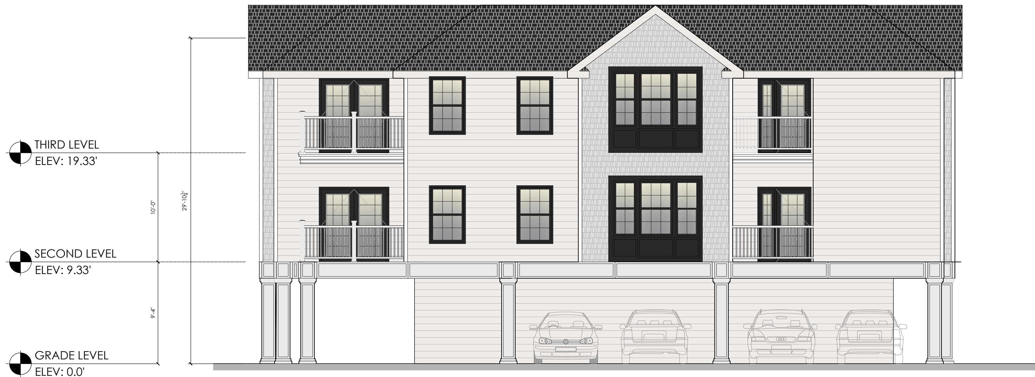
2 ELEVATION - SIDE (BLDG A) SCALE: 3/16" = 1'-0"
