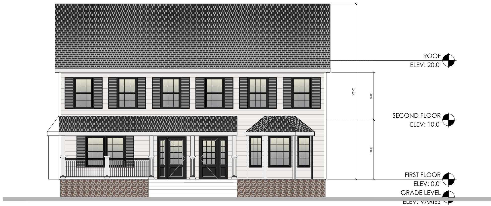
1 ELEVATION FRONT - TOWNHOUSE SCALE: 1/8" = 1'-0"
