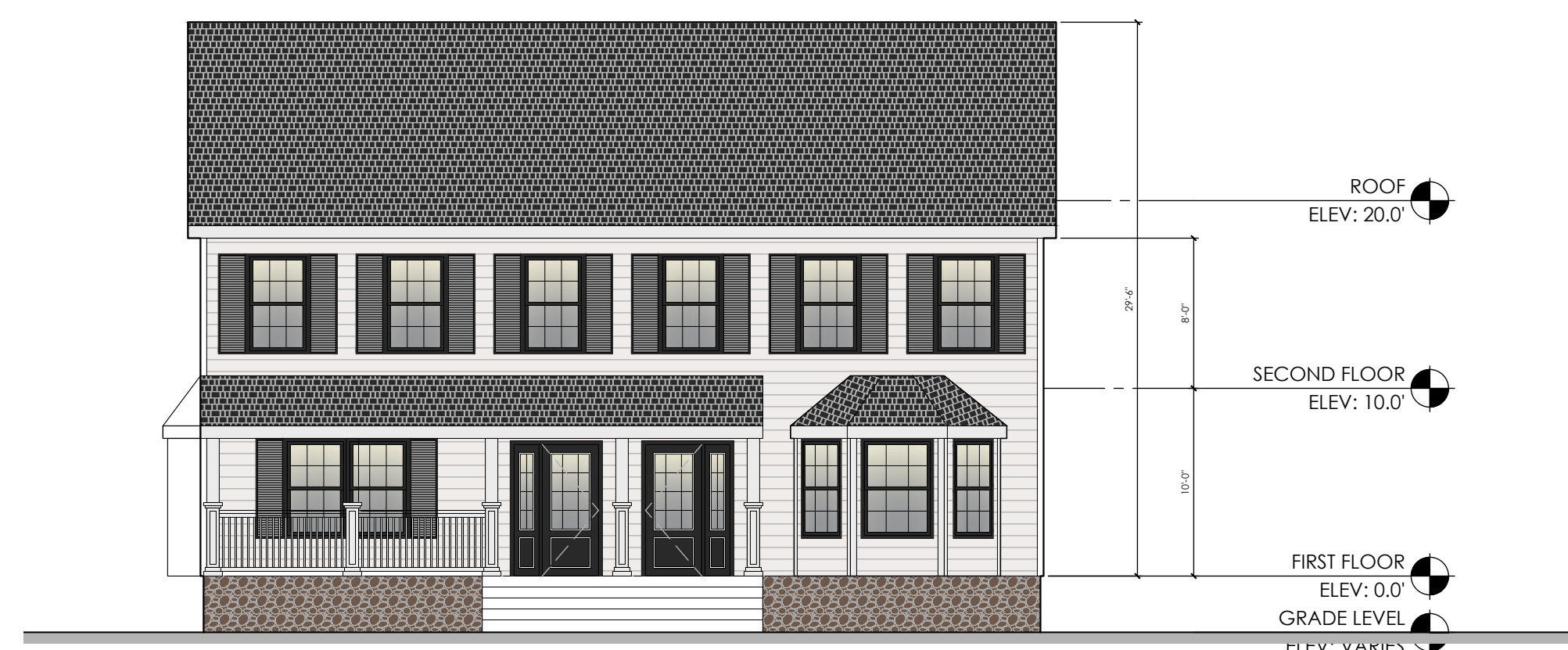
1 ELEVATION FRONT - TOWNHOUSE SCALE: 1/8" = 1'-0"
