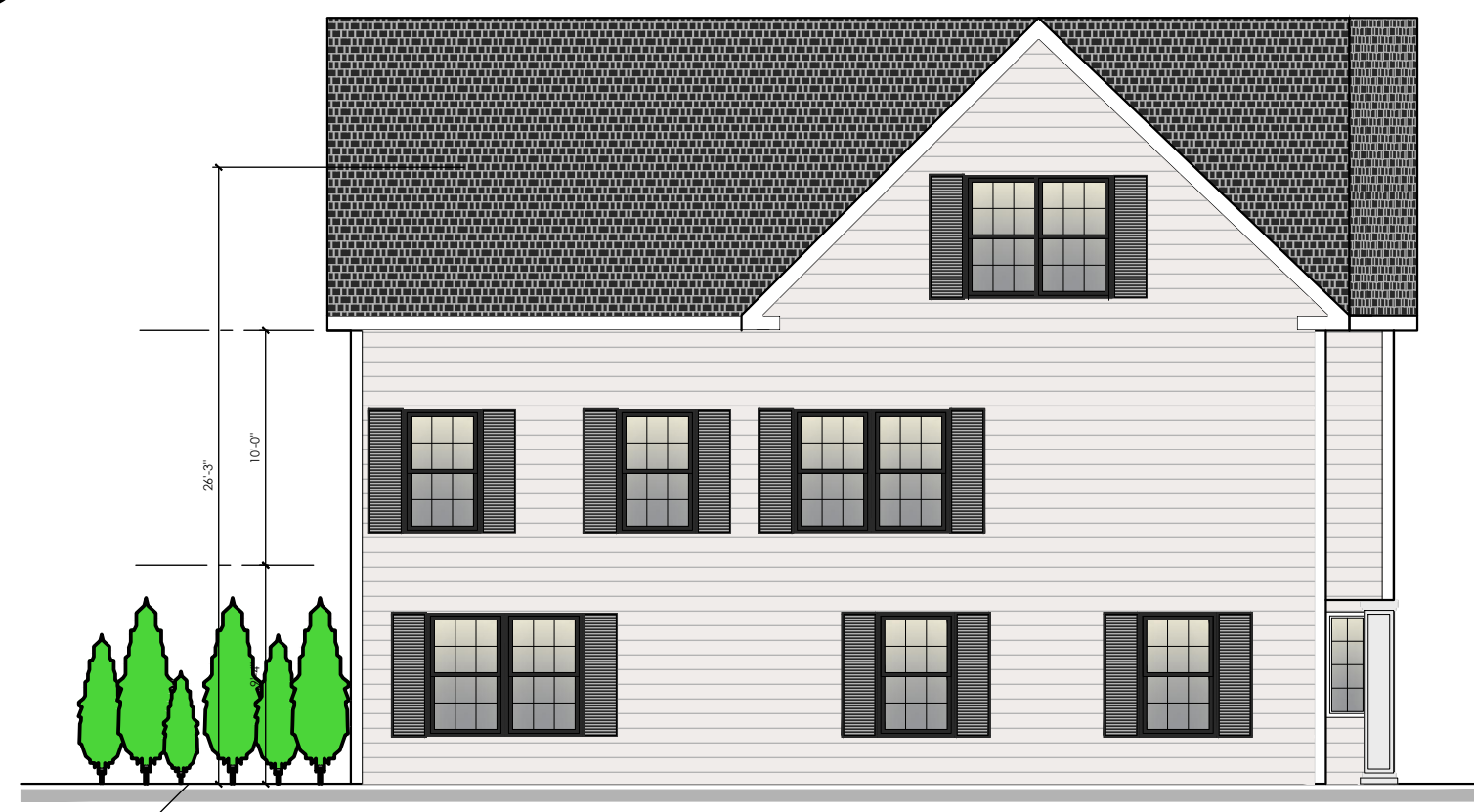
1 SIDE ELEVATION - TOWNHOUSE SCALE: 1/8" = 1'-0"
