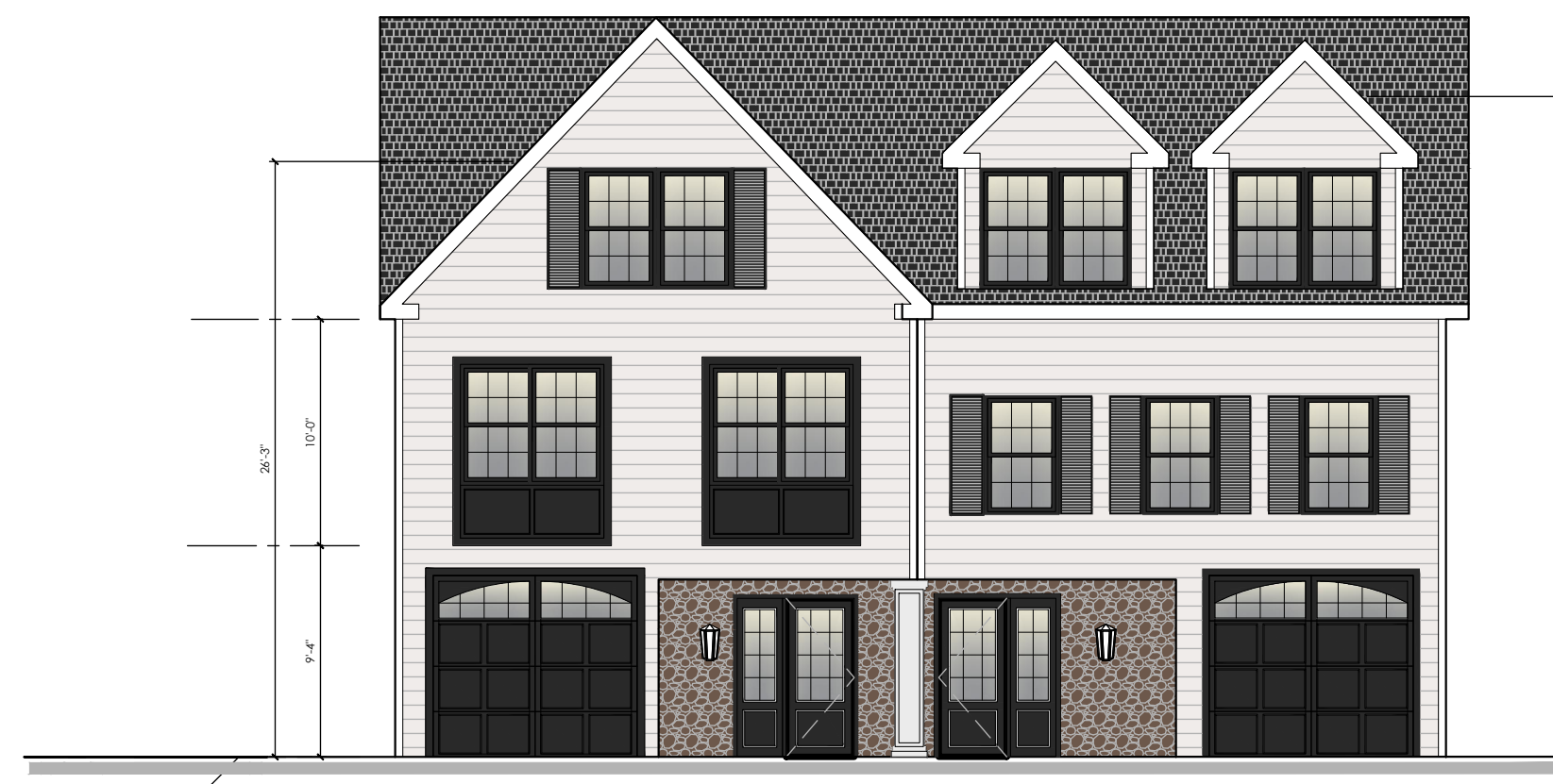
4 FRONT ELEVATION - TOWNHOUSE SCALE: 1/8" = 1'-0"
