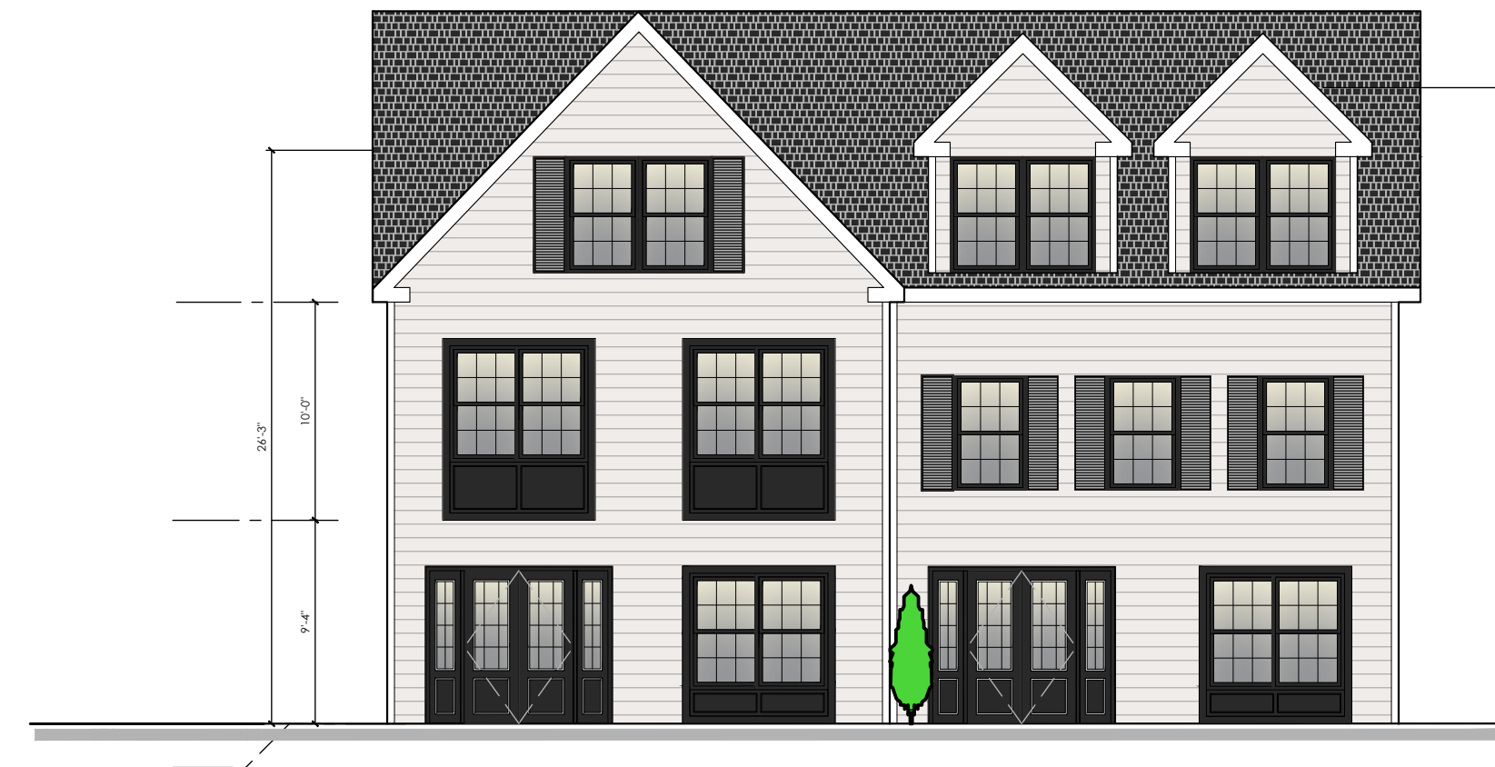
2 REAR ELEVATION - TOWNHOUSE SCALE: 1/8" = 1'-0"
