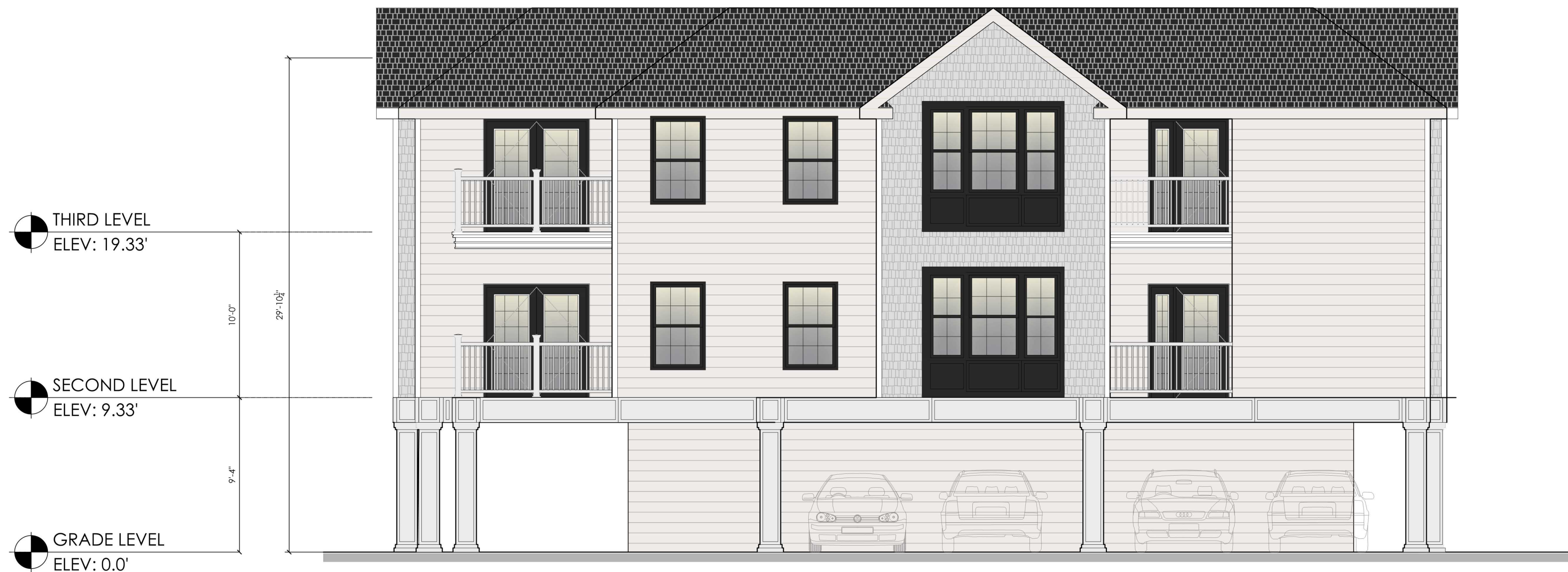
2 ELEVATION - SIDE (BLDG A) SCALE: 3/16" = 1'-0"
