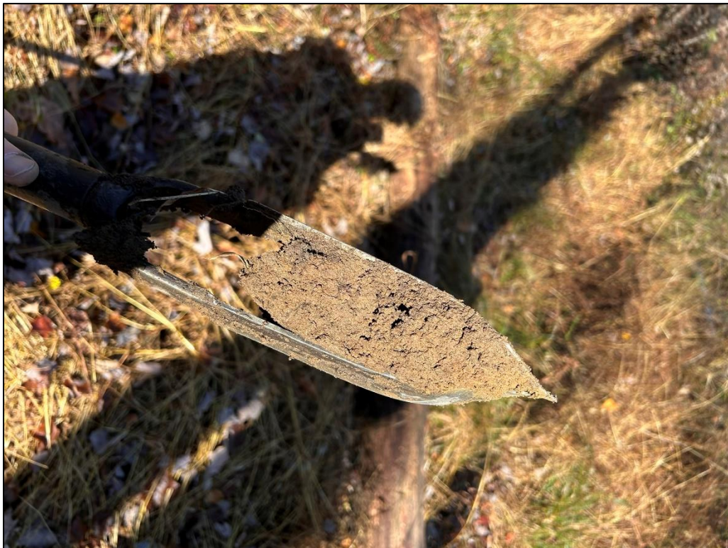
Photo 6. Showing standard non-hydric/oxidized soil which was found beneath an area which has “new” hydrology as described above.
