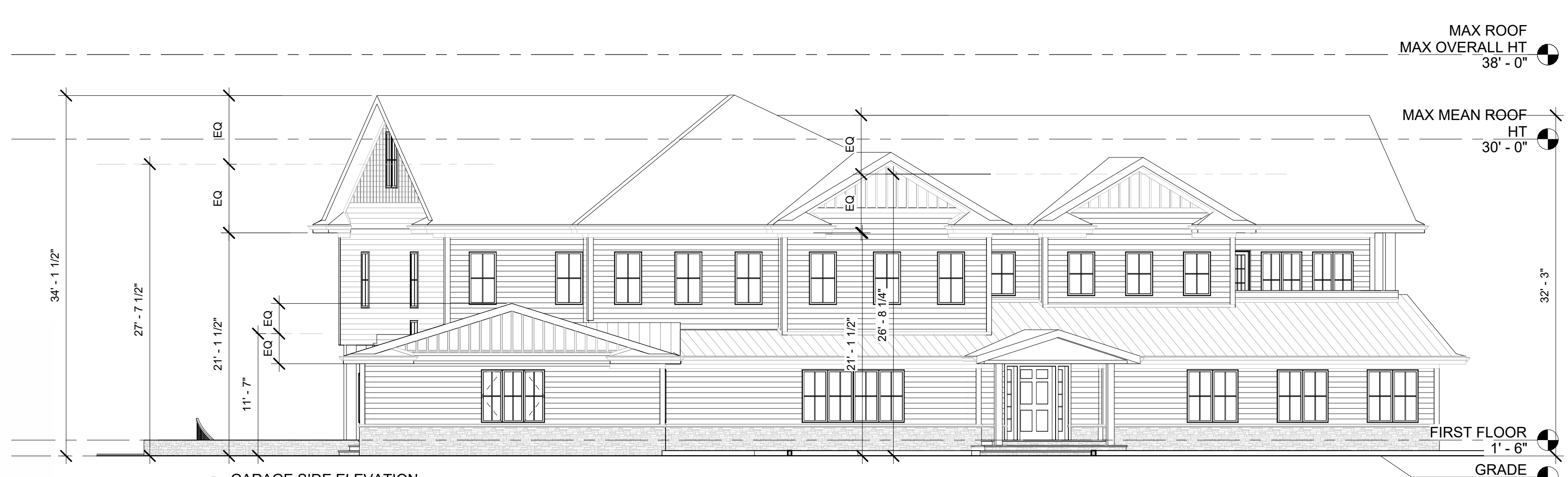
5 GARAGE SIDE ELEVATION 1/8" = 1'-0"
