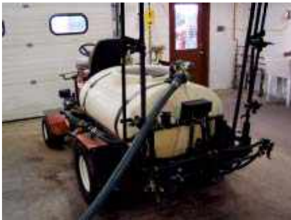
High volume transfer line and sprayer connections allow fast, spill free fill rates of 100 GPM or greater.
